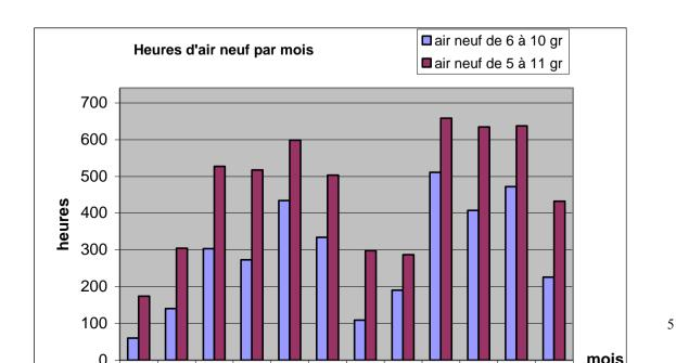
The graph above shows that the choice of the external conditions for shutting down the fresh airflow has serious consequences on the number of hours of ventilation.
