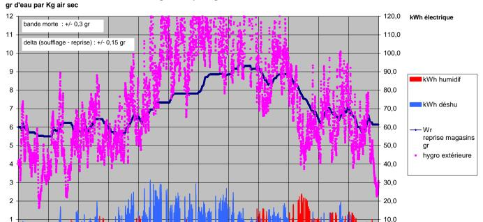
Hygrométrie absolue magasins gr d'eau par Kg air sec We should not let the lack of precision in humidity sensors reduce our optimism because we are not so much interested in the absolute value measured by the sensor as in its stability, i.e. its resolution and its repeatability in comparisons. The measurement will be off but it may be very stable.
