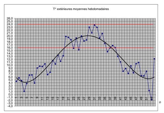
The need for air conditioning, excluding humidity treatment and compensation for possible internal contributions, can therefore be sharply reduced if we accept that the inside conditions are close to the 23/24°C zone.
